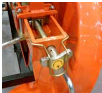
adjustable packing wheels to close & pack ground when plant comes out
