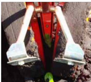
back kicker and front arm insures plant sets straight up
