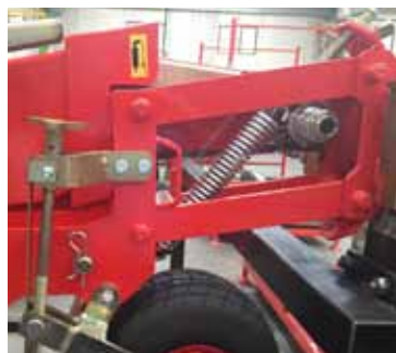
adjustable tension/parallelogram for constant planting depth
